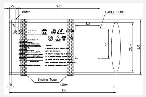
e) Silica Gel & Humidity Indicator Card inside Aluminum Vinyl Packing Bag
