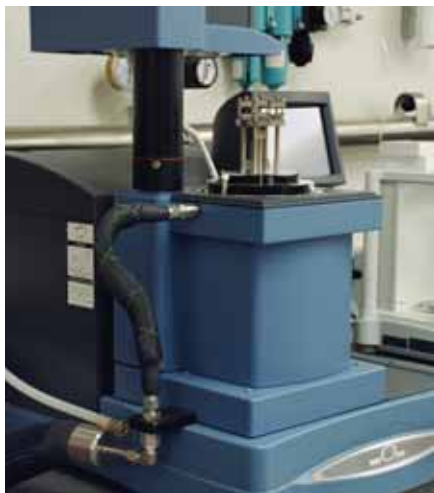
Dynamic Mechanical Analysis (DMA) – Measures the modulus of materials over a range of temperatures.
