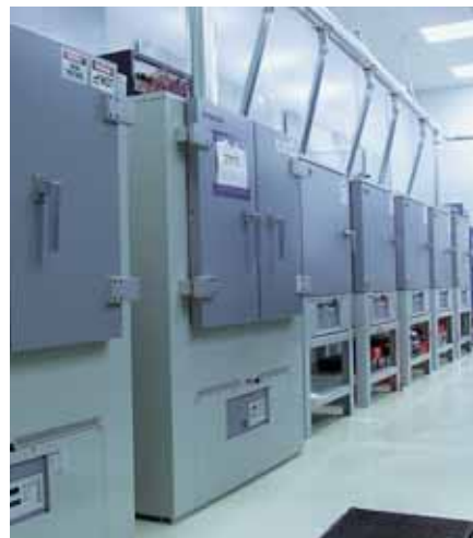
Chamber Ovens – Over 3000 cubic feet (85 cubic meters) of oven capacity is dedicated to long term thermal bias age testing. The ovens take material to temperatures above T_g . At selected intervals, samples are removed and tested to verify material integrity.
