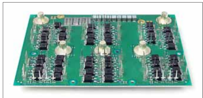
(48) FETs (9) Low profile capacitors (5) Low profile bus bars Total Weight 0.82 lbs (370.6 g)
