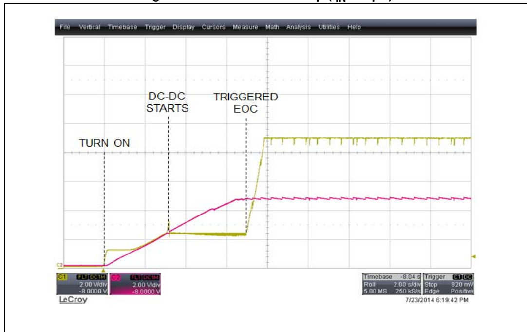
Figure 13. Buck-boost startup ( I_{IN} = 5 \mu A )
