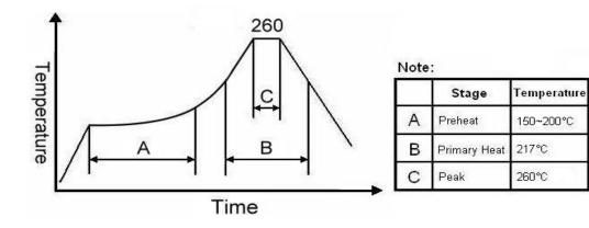
For soldering reflow profile and reliability test ratings go to: http://www.pericom.com/pdf/sre/reflow.pdf
