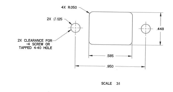
RECOMMENDED PANEL CUT OUT FOR HARDWARE INSTALLATION
