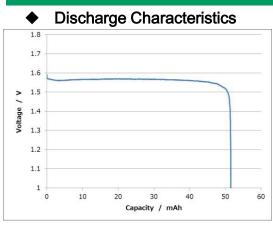
Measurement conditions: Temp: 23 deg C Load:  $15k\Omega$
