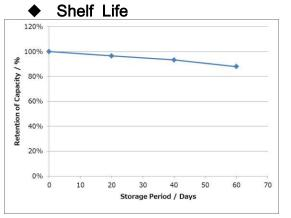
Measurement conditions:Temp:23 deg C Storage conditions: 60 deg C Dry Load:15kΩ
