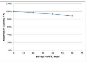
Measurement conditions:Temp:23 deg C Storage conditions: 60 deg C Dry Load: $15k\Omega$
