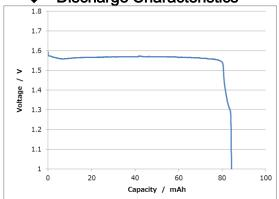
Measurement conditions: Temp: 23 deg C Load: 10kΩ
