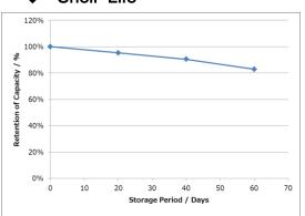
Measurement conditions: Temp: 23 deg C Storage conditions: 60 deg C Dry Load:100kΩ
