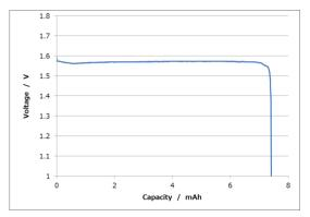
Measurement conditions: Temp: 23 deg C Load: 100kΩ
