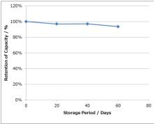
Measurement conditions:Temp:23 deg C Storage conditions: 60 deg C Dry Load:62kΩ
