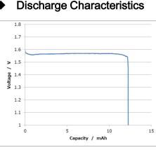
Measurement conditions: Temp: 23 deg C Load: 62kΩ
