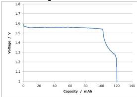
Measurement conditions: Temp: 23 deg C Load: 5.1kΩ
