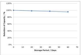
Measurement conditions:Temp:23 deg C Storage conditions: 60 deg C Dry Load:5.1kΩ
