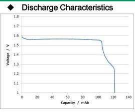
Measurement conditions: Temp: 23 deg C Load:  $5.1k\Omega$
