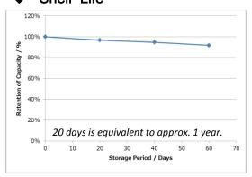
Measurement conditions:Temp:23 deg C Storage conditions: 60 deg C Dry Load:5.1k $\Omega$
