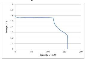
Measurement conditions: Temp: 23 deg C Load:  $5.1k\Omega$
