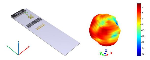
**3D pattern at 2.6 GHz**Drag to rotate pattern and PCB by using Adobe Reader
