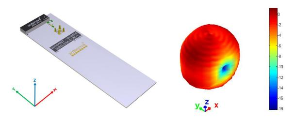
**3D pattern at 880 MHz**Drag to rotate pattern and PCB by using Adobe Reader
