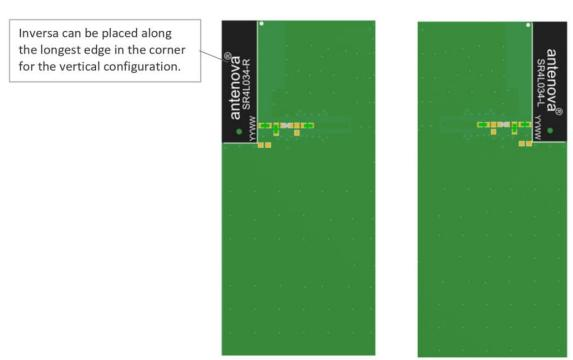
**Note:** Vertical placement optimal minimum GND length required is ≥100mm
