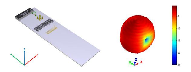
**3D pattern at 746 MHz**Drag to rotate pattern and PCB by using Adobe Reader
