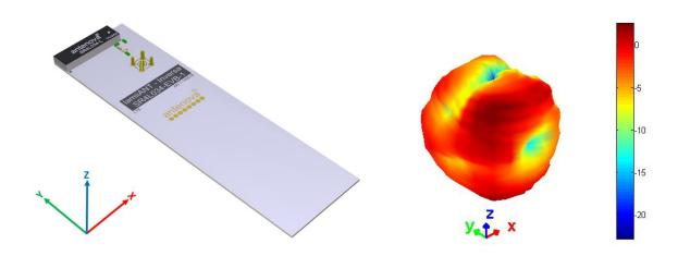
**3D pattern at 2.35 GHz**Drag to rotate pattern and PCB by using Adobe Reader
