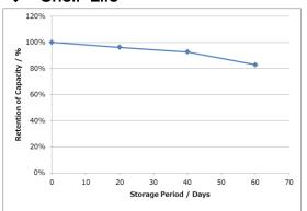
Measurement conditions:Temp:23 deg C Storage conditions: 60 deg C Dry
