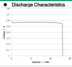
Measurement conditions: Temp: 23 deg C Load: 62 k $\Omega$
