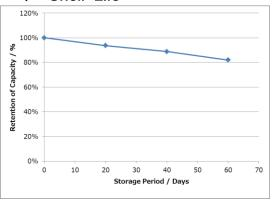
Measurement conditions:Temp:23 deg C Storage conditions: 60 deg C Dry Load: $36k\Omega$
