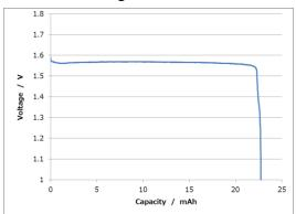
Measurement conditions: Temp: 23 deg C Load:  $36 \text{ k}\Omega$
