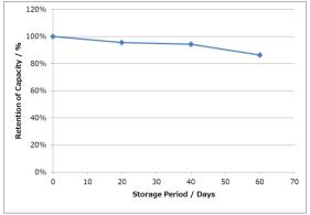
Measurement conditions:Temp:23 deg C Storage conditions: 60 deg C Dry Load: $43k\Omega$
