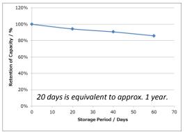
Measurement conditions:Temp:23 deg C Storage conditions: 60 deg C Dry Load:30kΩ
