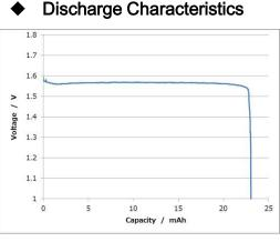
Measurement conditions: Temp: 23 deg C Load: 30kΩ
