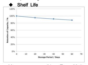
Measurement conditions:Temp:23 deg C Storage conditions: 60 deg C Dry Load:24kΩ
