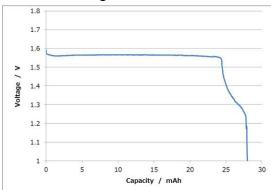
Measurement conditions: Temp: 23 deg C Load: 24kΩ
