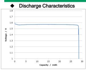
Measurement conditions: Temp: 23 deg C Load: 24 k $\Omega$
