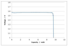
Measurement conditions: Temp: 23 deg C Load:  $82k\Omega$
