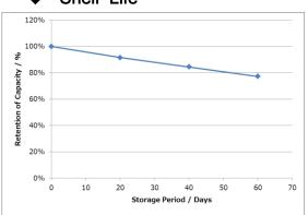
Measurement conditions:Temp:23 deg C Storage conditions: 60 deg C Dry Load: $82k\Omega$
