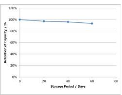
Measurement conditions:Temp:23 deg C Storage conditions: 60 deg C Dry Load: $36k\Omega$
