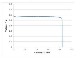
Measurement conditions: Temp: 23 deg C Load:  $36k\Omega$
