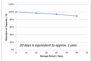
Measurement conditions:Temp:23 deg C Storage conditions: 60 deg C Dry
