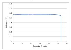
Measurement conditions: Temp: 23 deg C Load: 30kΩ
