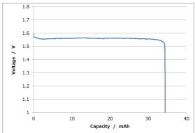
Measurement conditions: Temp: 23 deg C Load:  $20k\Omega$
