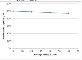
Measurement conditions:Temp:23 deg C Storage conditions: 60 deg C Dry Load: $24k\Omega$
