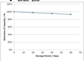
Measurement conditions:Temp:23 deg C Storage conditions: 60 deg C Dry Load: $20k\Omega$
