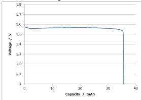
Measurement conditions: Temp: 23 deg C Load: 20kΩ
