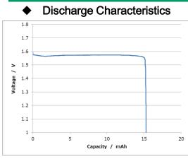
Measurement conditions: Temp: 23 deg C Load:  $62k\Omega$
