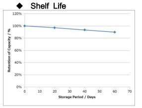
Measurement conditions:Temp:23 deg C Storage conditions: 60 deg C Dry Load:62kΩ
