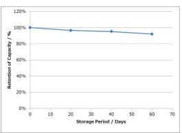
Measurement conditions: Temp: 23 deg C Storage conditions: 60 deg C Dry Load:30kΩ
