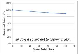
Measurement conditions:Temp:23 deg C Storage conditions: 60 deg C Dry Load:20kΩ
