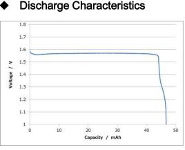
Measurement conditions: Temp: 23 deg C Load: 20kΩ
