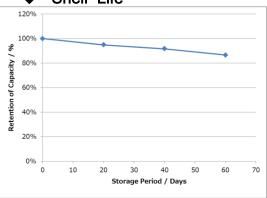
Measurement conditions:Temp:23 deg C Storage conditions: 60 deg C Dry Load: $15k\Omega$
