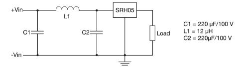
C1, C2 and L1 should be placed as close to the SRH05 as possible
