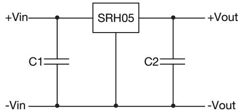
C1 = 3.3  $\mu$ F/100 V required if input voltage is above 50 VDC
