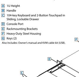
The SRSHELFKBD SmartRack® 1U Rack-Mount Keyboard is a full 104-key keyboard and two-button touchpad designed for mounting in an EIA-standard 19-inch rack. It can be mounted in a 2- or 4- post rack. Tripp Lite's B019-000 bracket (sold separately) is required for two-post mounting. It's ideal for use with KVM switches and servers that don't include a keyboard.
