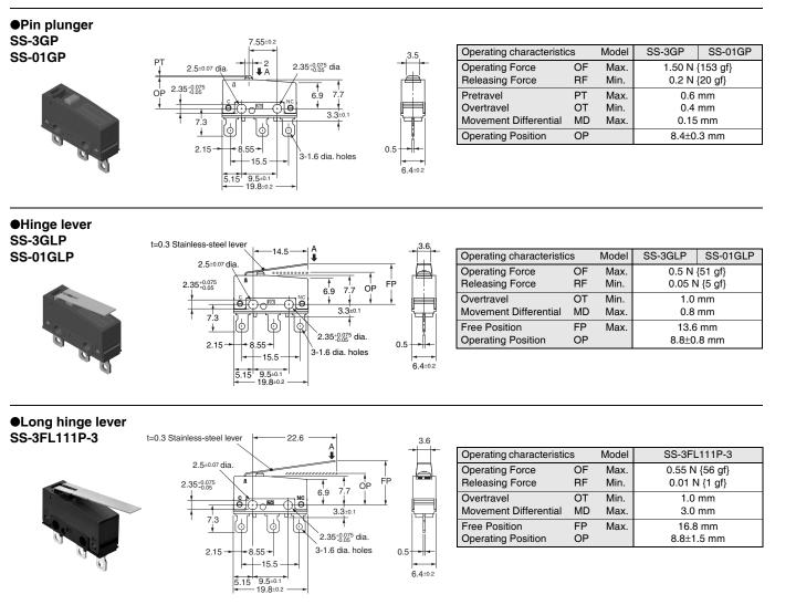
Note 1. Unless otherwise specified, a tolerance of  $\pm 0.4$  mm applies to all dimensions. Note 2. The operating characteristics are for operation in the A direction (  $\clubsuit$  ).
