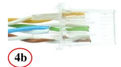
First insert Org, Grn, Brn pairs into lower row of load bar, then insert Blu into upper row
