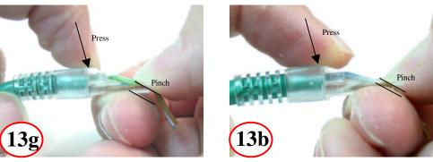
Pinch load bar end, then press on back to set wires in place
