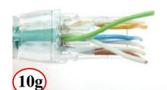
Check Grn pair for alignment Add ½ twist if necessary
