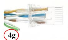
First insert Org, Blu, Brn pairs into lower row of load bar, then insert Grn into upper row
