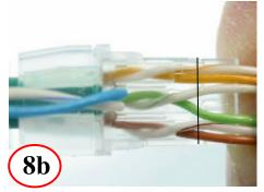
Untwist lower three pairs back to ends of side walls. Spread Grn pair
