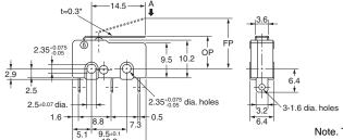
Note. The indicated reference values of RF are for cases where the lever weight is not applied to the plunger.
