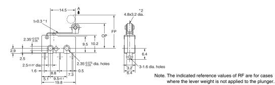
\*1. Stainless-steel lever \*2. Polyacetal resin roller
