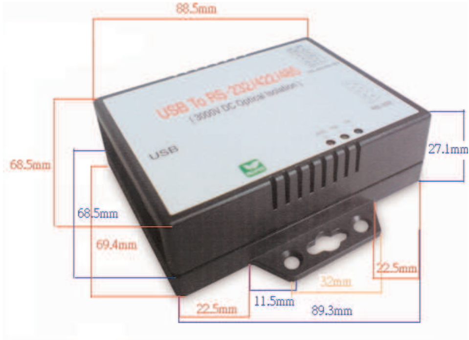
SSU2-400I- Single port RS-232/422/485 USB Serial Adapter with optical isolation
