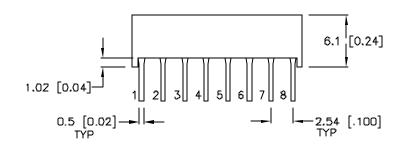
UNIT: mm [INCHES] TOLERANCE:  $\pm 0.25$  [ $\pm 0.01$ ] UNLESS OTHERWISE SPECIFIED
