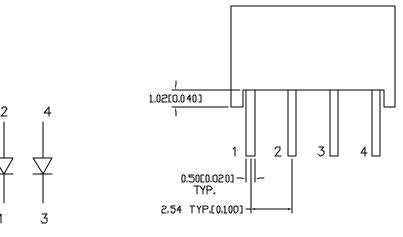
UNIT: mm (INCHES) TOLERANCE  $\pm 0.25$  ( $\pm 0.01$ ) UNLESS OTHERWISE SPECIFIED
