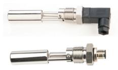
The SSF212 series are horizontally mounted switches that are fitted via a  $\frac{1}{2}$ "NPT thread from the outside of the tank, so does not require access to the inside of the tank.
