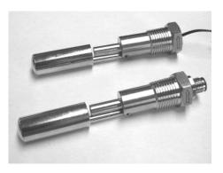
The SSF215 series of floatswitches are externally mounted horizontal switches. This series has an extended reach to provide a solution for extra thick tank walls or for mounting in welded on 1/2"NPT bosses.
