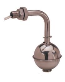
The SSF29 type is a side mount vertical switch designed to give reliable switching at higher pressures, up to 40 bar. The switch is mounted in the side of the tank, from the inside, so requires access to the inside of the tank.
