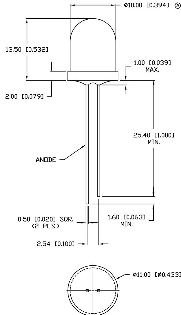
UNLESS OTHERWISE SPECIFIED TOLERANCE IS  $\pm .25\text{mm}$  ( $\pm 0.010"$ )
