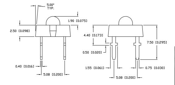
UNLESS OTHERWISE SPECIFIED TOLERANCE IS ±.25mm (±0.010")
