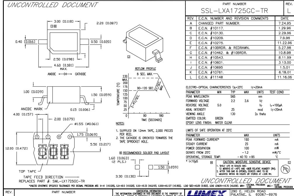
SSL-LXA1725GC-TR AXIAL LEAD WITH FLAT TOP AND MOLDED REFLECTOR, 565nm GREEN LED, WATER CLEAR LENS, TAPE AND REEL.
