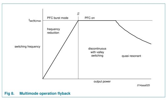
At high output power the converter switches to quasi-resonant mode. The next converter stroke is started after demagnetization of the transformer current. In quasi-resonant mode switching losses are minimized as the converter only switches on when the voltage across the external MOSFET is at its minimum (valley switching, see also Section 7.3.2).
