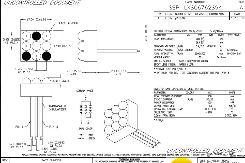
0.67" SQUARE, 9 LAMP POLYLED, COMMON ANODE, RED/GREEN LEDS, WATER CLEAR LENS.
