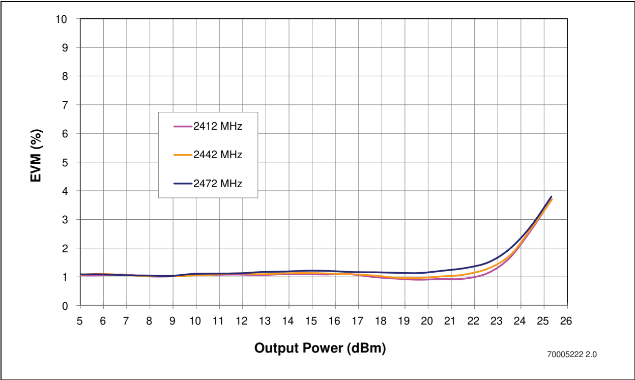
FIGURE 5-3: DYNAMIC EVM VERSUS OUTPUT POWER 802.11AC, MCS9-VHT40, 50% DUTY CYCLE
